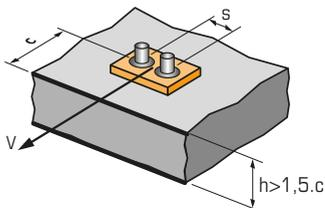
$$\Psi_{s-c,V} = \frac{3 \cdot c + s}{6 \cdot c_{min}} \cdot \sqrt{\frac{c}{c_{min}}}$$
