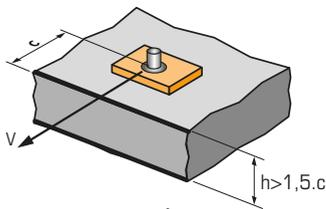
$$\Psi_{s-c,V} = \frac{c}{c_{min}} \cdot \sqrt{\frac{c}{c_{min}}}$$
